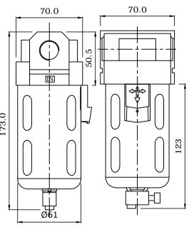
•Supply pressure 6 bar , pressure drop p=0.3 bar ( for standard models ).
